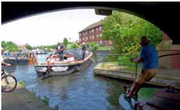
In Liverpool, Alan Holden with **Anna** towed **Kennet** backwards to the end of the canal as there is not enough width to turn there. The canal is also shallow here, which makes travelling in reverse a problem as stirring up the bottom results in **Kennet's** cooling water inlet becoming blocked.
