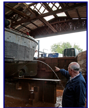
There was a "hole in our ballast tank"
